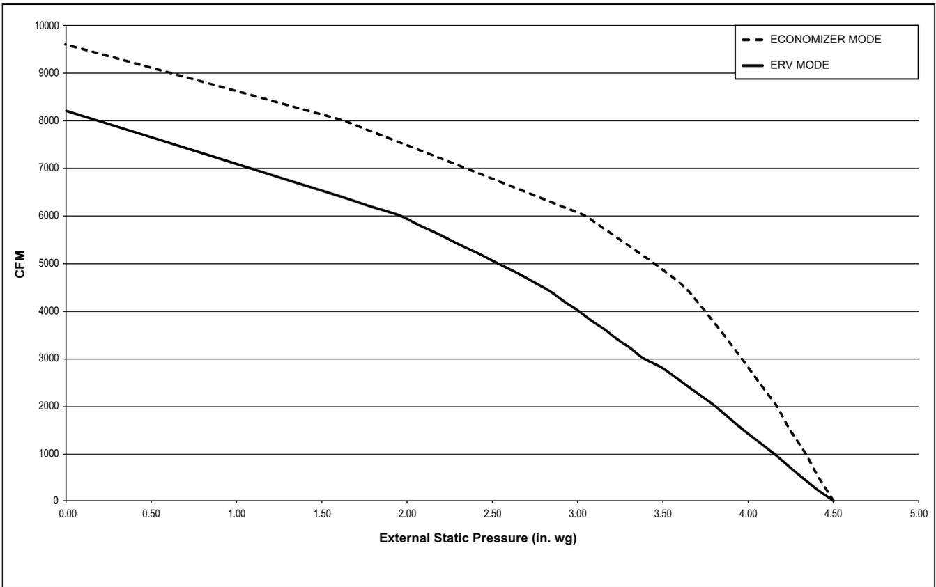
**Fig. 17 - 50HC\*\*28 Supply and Exhaust Fan Performance Curves**
