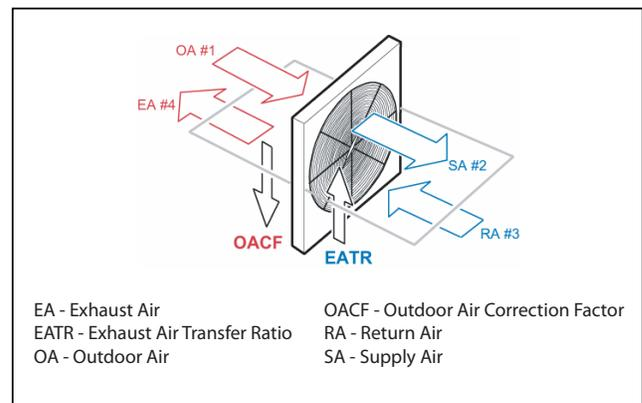
Fig. 19 - Air-to-Air Energy Recover Ventilation - Airflow Convention
