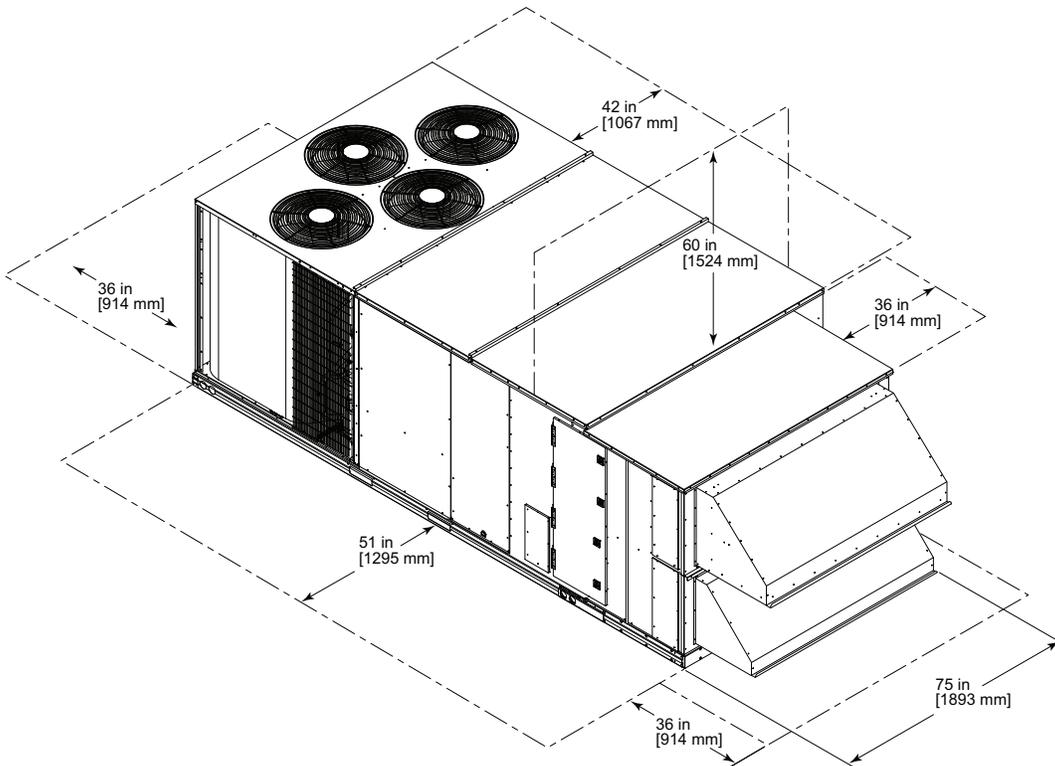
**Fig. 10 - Clearances for ERV on Size 24 & 28 Base Units**
