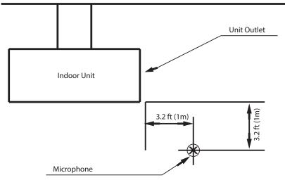
Fig. 7 – Sound Pressure Testing Method
