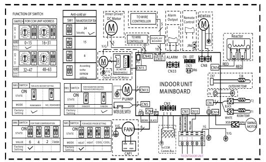
Fig. 8 – Wiring Diagram (Sizes 9K-24K)
