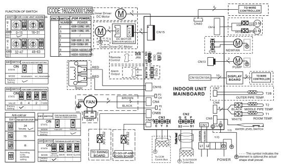
Fig. 9 – Wiring Diagram (Size 36K–48K)
