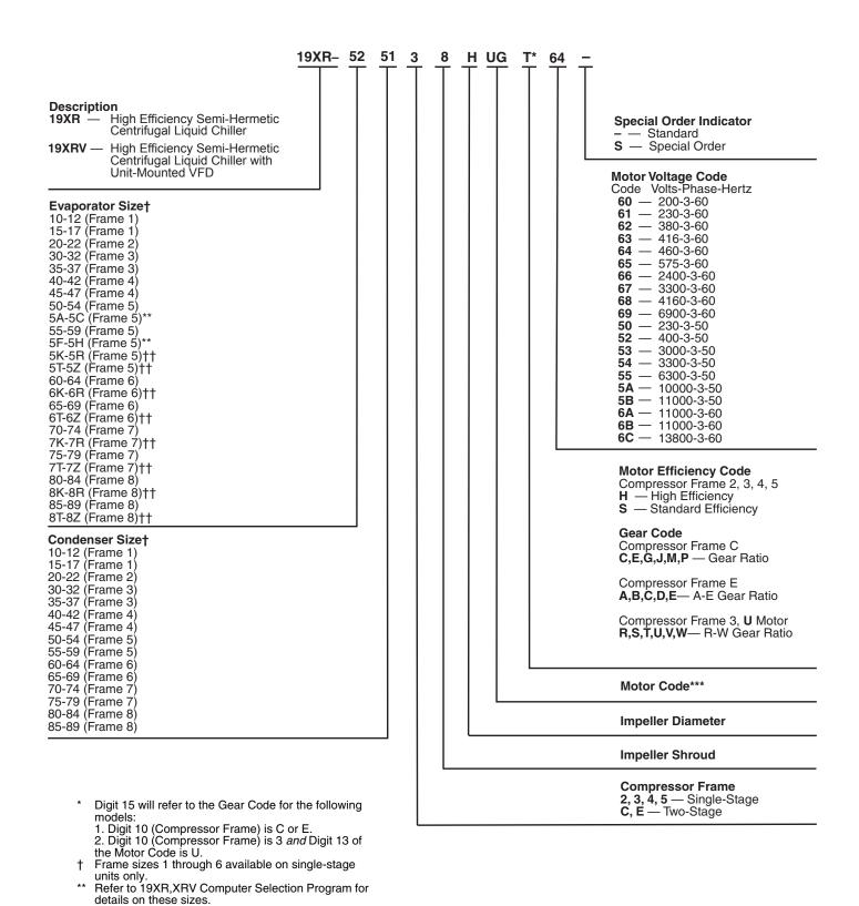
Fig. 2 — 19XR,XRV Single-stage Compressor and Two-stage Compressor Frame Size C and E
