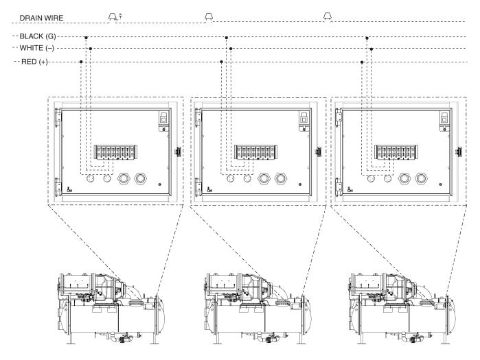
NOTE: Field-supplied terminal strip must be located in control panel.
