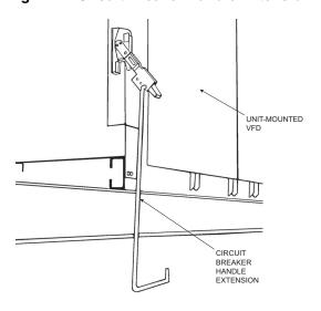
Fig. 48 — Circuit Breaker Handle Extension Installed
