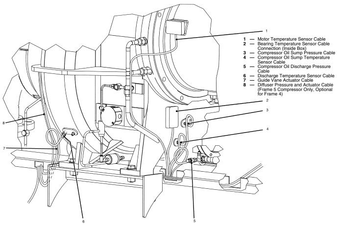
Fig. 19 — Compressor Detail
