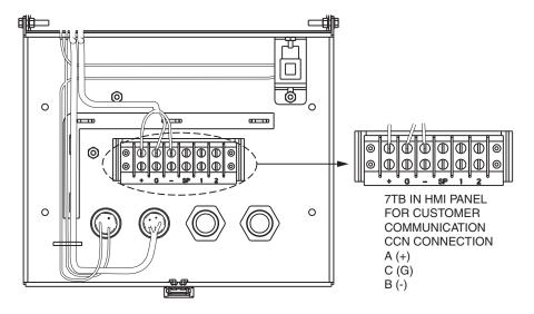
Fig. 53 — 19XR6/7 HMI Panel
