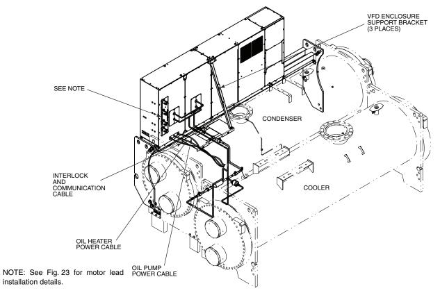
Fig. 22 — 900A or 1200A LF2 VFD or Standard Tier VFD (765, 855, 960, 1070, 1275, 1530A) Installation — Typical
