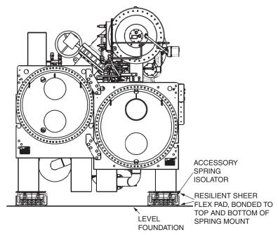
NOTE: The accessory spring isolators are supplied by Carrier for installation in the field if the accessory is purchased.
