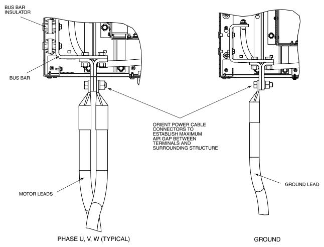
Fig. 25 — Motor Lead Installation (View Looking Down)
