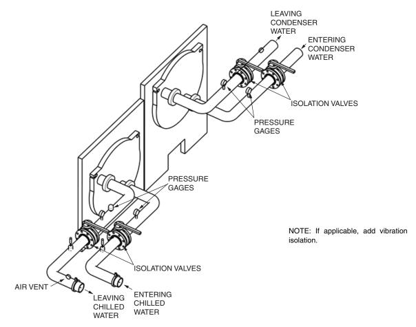
Fig. 38 — Typical Nozzle Piping
