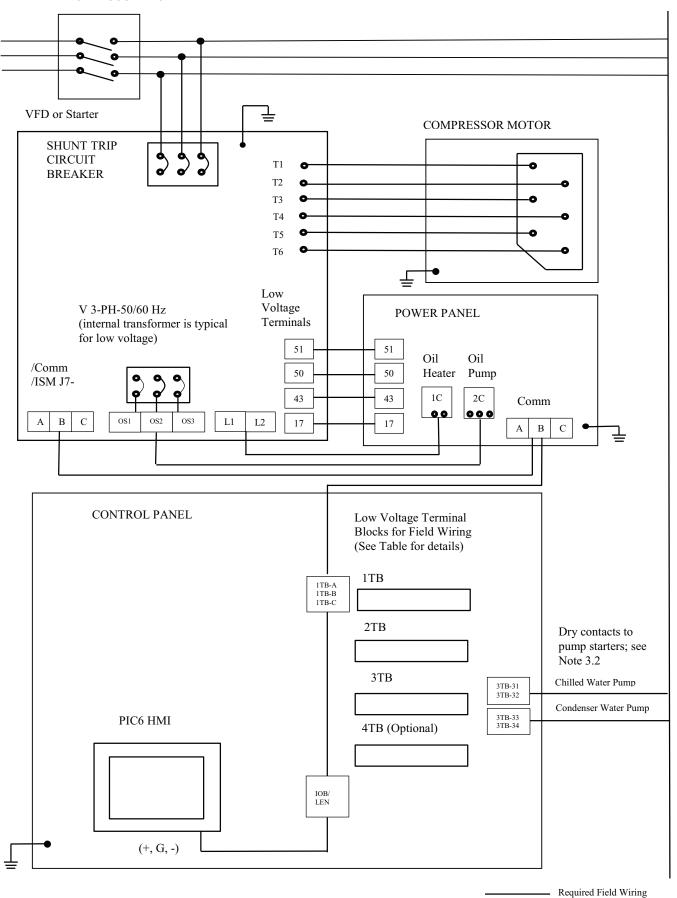
Fig. 57 — Typical 19XR2-E Fixed Speed or VFD — Factory Unit Mounted (Low Voltage)
