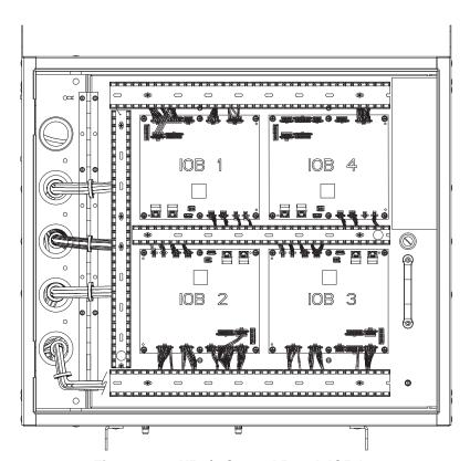
Fig. 54 — 19XR6/7 Control Panel, IOB Layer
