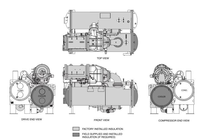
Fig. 70 — 19XR Insulation Area (Typical Unit with Economizer)
