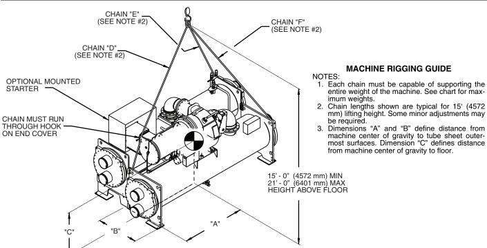
Fig. 9 — Machine Rigging Guide (Heat Exchanger Size 10 Through 7R) with Free-Standing or Unit-Mounted Starter
