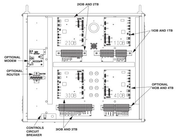
Fig. 51 — 19XR2-E Control Panel Layout and Field Connections
