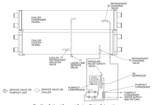
Fig. 43 — Optional Pumpout System Piping Schematic
