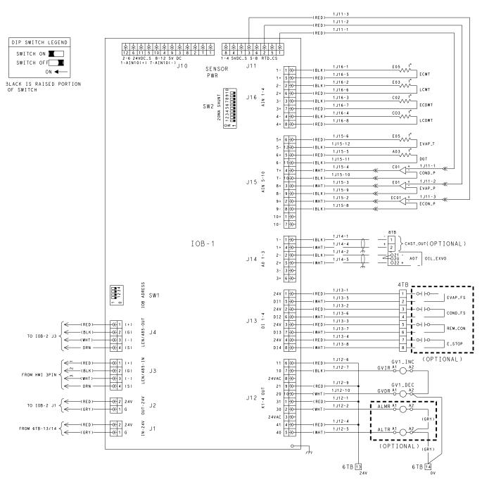
Fig. 67 — 19XR6-7 Chiller Control Schematic
