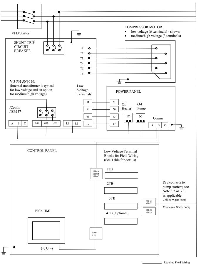
Fig. 59 — 19XR2-E with Free-Standing Low Voltage Starter; 19XR2-E with Free-Standing Low Voltage VFD; 19XR2-E with Free-Standing Medium Voltage Starter with Integrated Starter Module (ISM)
