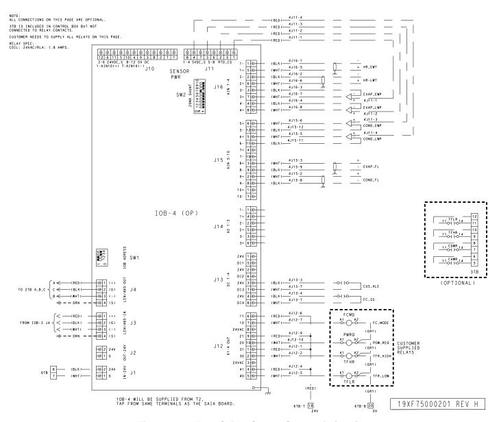
Fig. 67 — 19XR6-7 Chiller Control Schematic (cont)
