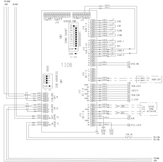
Fig. 61 — 19XR2-E Chiller Control Schematic FIELD TERMINALS for 1TB, Fig. 61
