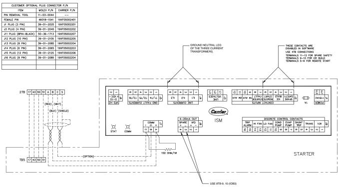
NOTE: For medium voltage free-standing VFD, TB5 is identified as drive terminal block 1 and is located at the low voltage terminal strip.
