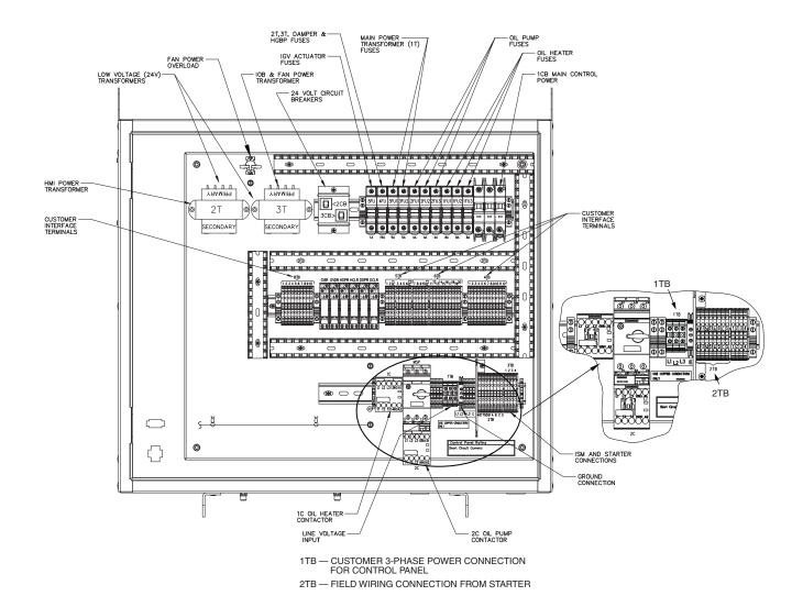
Fig. 55 — 19XR6/7 Control Panel, Bottom Layer
