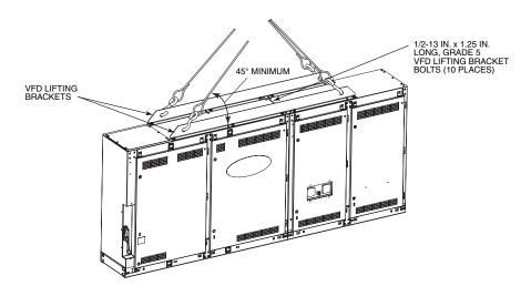
Fig. 27 — 900A or 1200A VFD Enclosure Lifting Points
