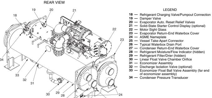
Fig. 5 — 19XR,XRV Two-Stage Compressor Frame Size C and E
