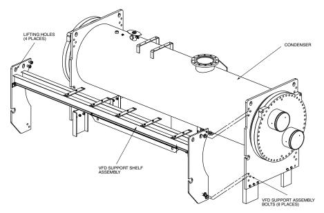
Fig.  $28 - 900 \mathrm{A}$  or 1200 A VFD Support Assembly Installation
