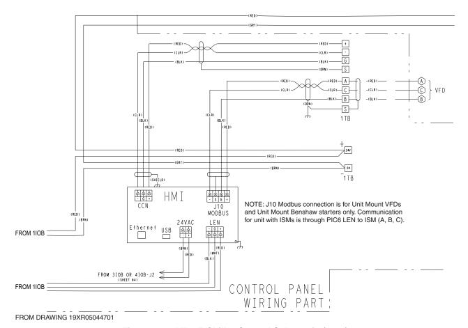
Fig. 61 — 19XR2-E Chiller Control Schematic (cont)
