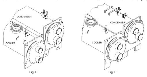
Fig. 44 — 19XRV Relief Valve Arrangements
