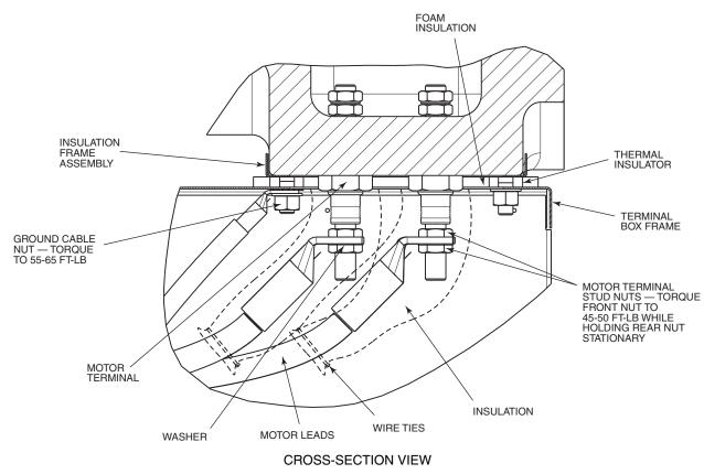
Fig. 24 — Compressor Motor Terminals (Typical)
