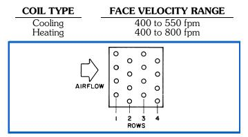
In variable air volume (VAV) applications, the system generally operates below peak air volume for extended periods. In such cases, the design face velocity is commonly selected at the higher end of the suggested range.
